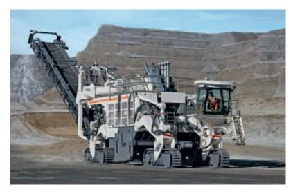
Due to the simultaneous work processes of cutting, crushing and loading, material extraction using Wirtgen Surface Miners is particularly efficient. Worldwide mining companies and mine operators are exploiting the advantages of this technology. Due to the precise control of the cutting depth the machine can be optimally adjusted to the prevailing conditions, for example on cutting seams, intermediate layers or extracting high quality material such as coal, phosphate, and gypsum.
