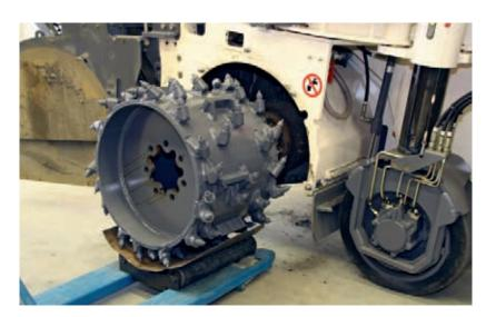
The centring bolts for FCS milling drums make it possible to quickly and straightforwardly change the milling drums. To adjust the milling drum with the aid of a carriage or fork lift truck on the gearbox, it is recommended to use two centring bolts.
