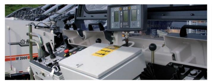
To be able to retrofit older series with the innovative grade and slope control system LEVEL PRO, Wirtgen offers retrofit kits with which the conversion to the new system can be made quickly and straightforwardly.
