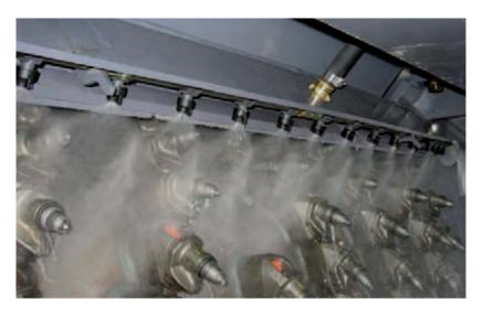
The different spray units at a variety of different locations on the road milling machine – such as on the bottom conveyor, in the transfer area from the bottom conveyor to the top one, or in the milling drum housing – ensure adequate and even distribution of a spraying mist that cleans all the components.
