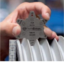
Belt pulleys profile gauge Part No.: 2065403
