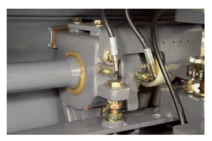
Given a maximum tamper speed of 1,800 rpm and the beating action of the tamper bars, tamper bearings are exposed to highest continuous strain. This is why we use bearings and bearing housings of prime quality only and tolerances for manufacture are extremely tight.
