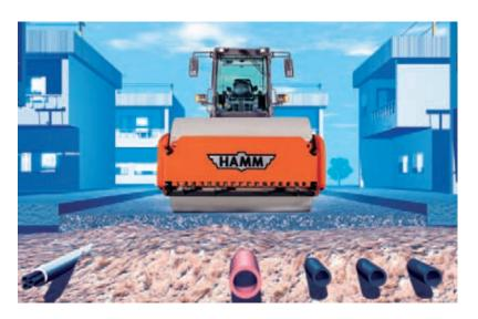
For earth compactors there is also the possibility for the oscillation compaction, here is the VIO drum used. In this drum both systems are combined, so that there can be selected between oscillation and vibration.
