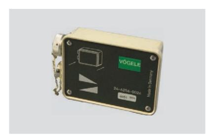
The Big MultiPlex Ski comes with 3 sonic grade sensors. Each of them has 5 sensing cells picking up actual values over a length of 28 cm. For calculating an average, however, only three measurements are used out of five, in fact those showing the smallest deviation from the value specified.
