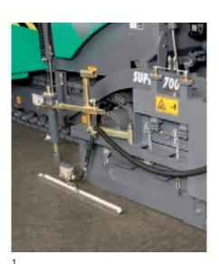
1 Referencing with mechanical grade sensor and ski.
