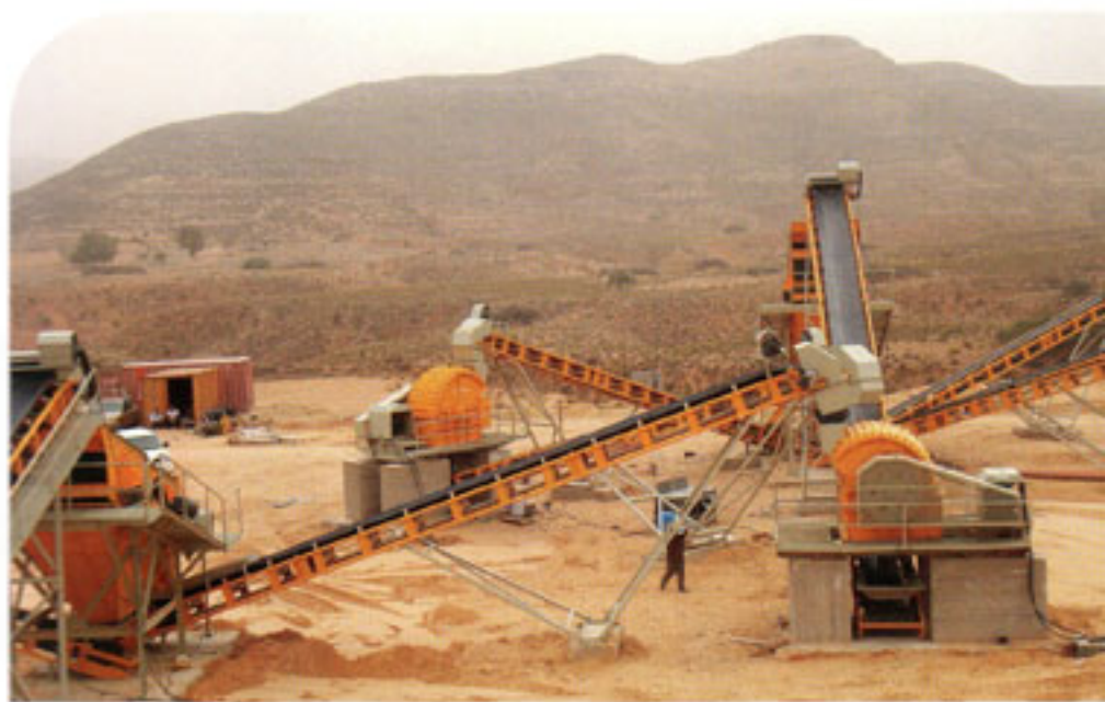
With its crushing, sieving, conveying and washing machines, Seytas is also active in other countries of the Middle East and in North Africa.
